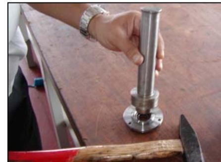
*Insert until stop the oil seal, using a insertion punch and
